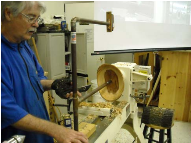
Measuring wall thickness using laser light.
