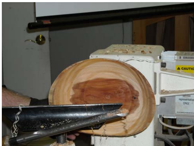
Getting the right curvature. Look for gaps by using a ruler or straightedge.
