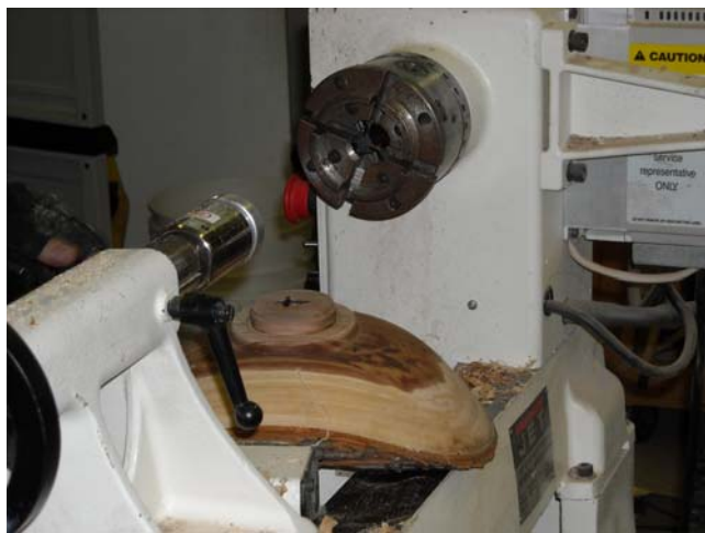
Getting the right curvature. Look for gaps by using a ruler or straightedge.
